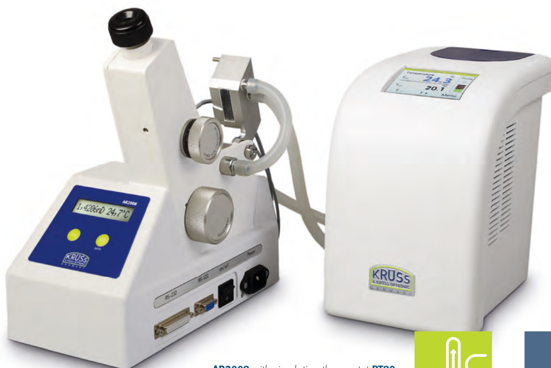
AR2008 with circulating thermostat PT80
